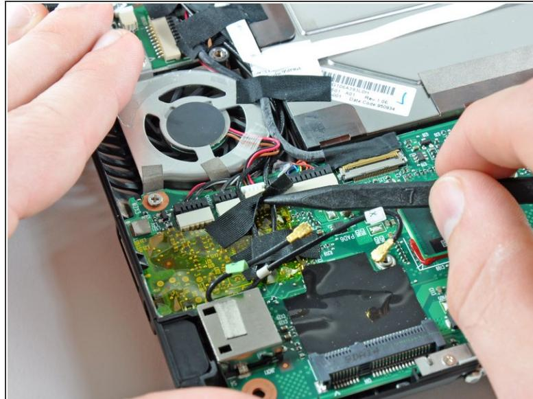
ⓘ If present, remove the pieces of black cloth tape securing the antenna cables to the motherboard.
