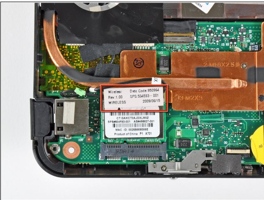
ⓘ If present, peel the sticker up off the top of the Wi-Fi board to reveal the Wi-Fi antenna connectors.
