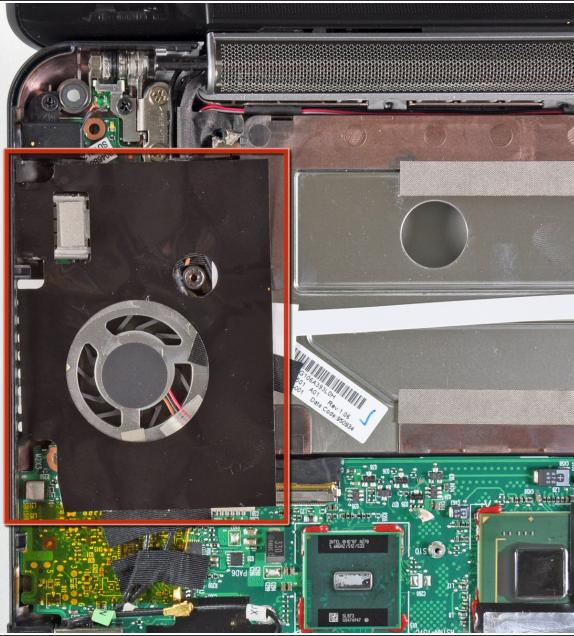
ⓘ If present, remove the large piece of black adhesive film covering the area around the fan.
