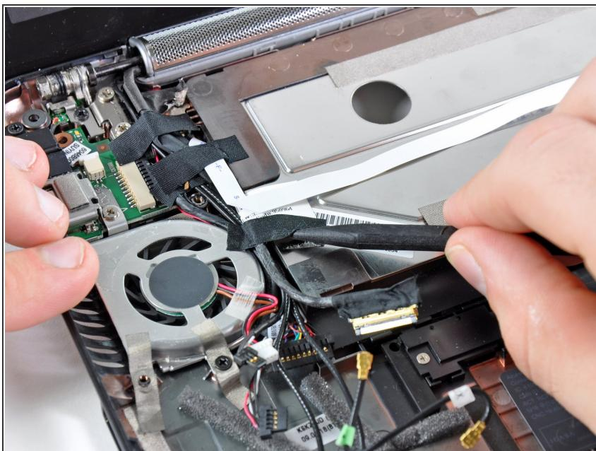
ⓘ If present, remove the piece of black cloth tape holding the bundle of cables to the top of the fan.
