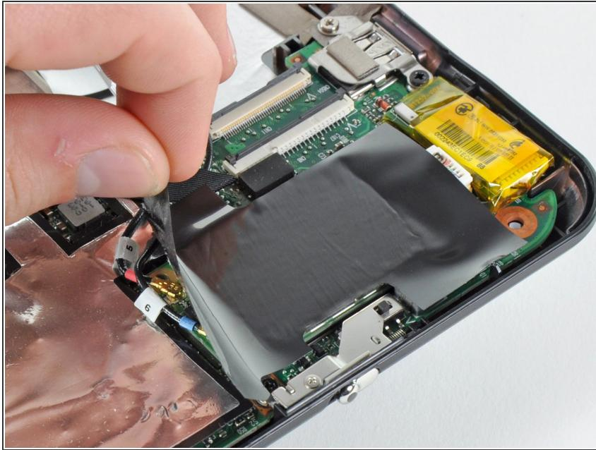
ⓘ If present, carefully peel the piece of tape covering the WWAN board.
